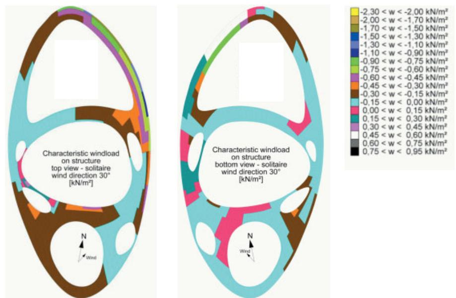
Fig. 3. Example for wind load distributions
