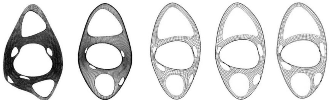
Fig. 5. Evolution of the roof shape during form finding
