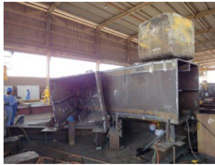
Fig. 16. Prefabrication of welded segments in the shop (left: compression ring, right: crossing point tension ring)
