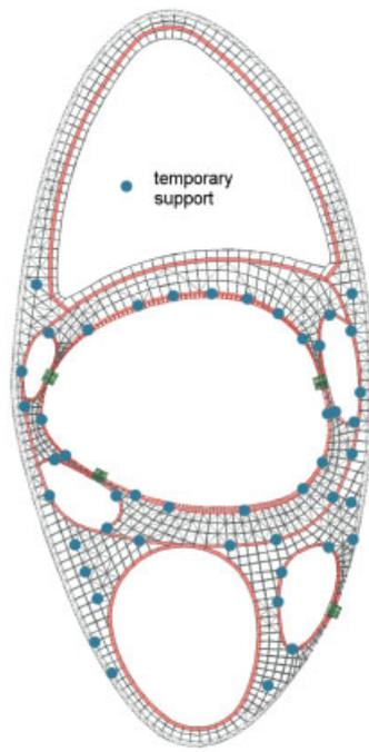
Fig. 11. Arrangement of temporary supports (trestles)
