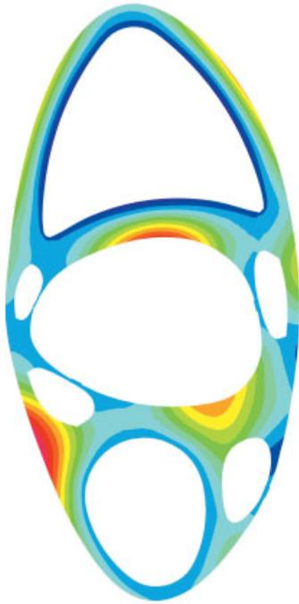
Fig. 10. Vertical deformations under dead load
