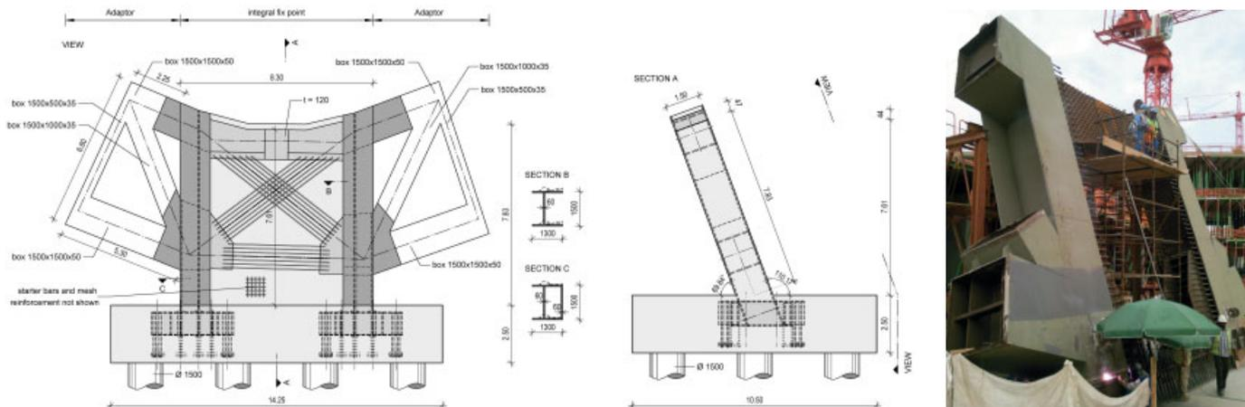
Fig. 8. Drawings and assembly of integral fix point
